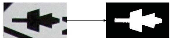
Fig. 6: Left to right: A jamdani motif image at the left and result of binarizing after applying opening and cropping operations.
